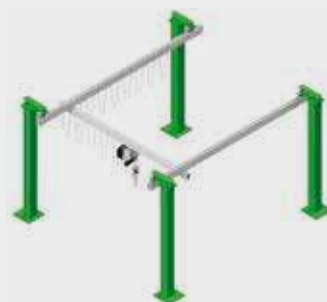
Bridge crane column mounted
